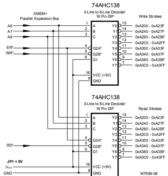
Figure 7 - Write / Read Decoder Circuitry
