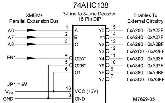
Figure 6 - Address Decoder
