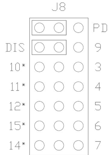
**Figure 4 - J8 Interrupts Configuration**
