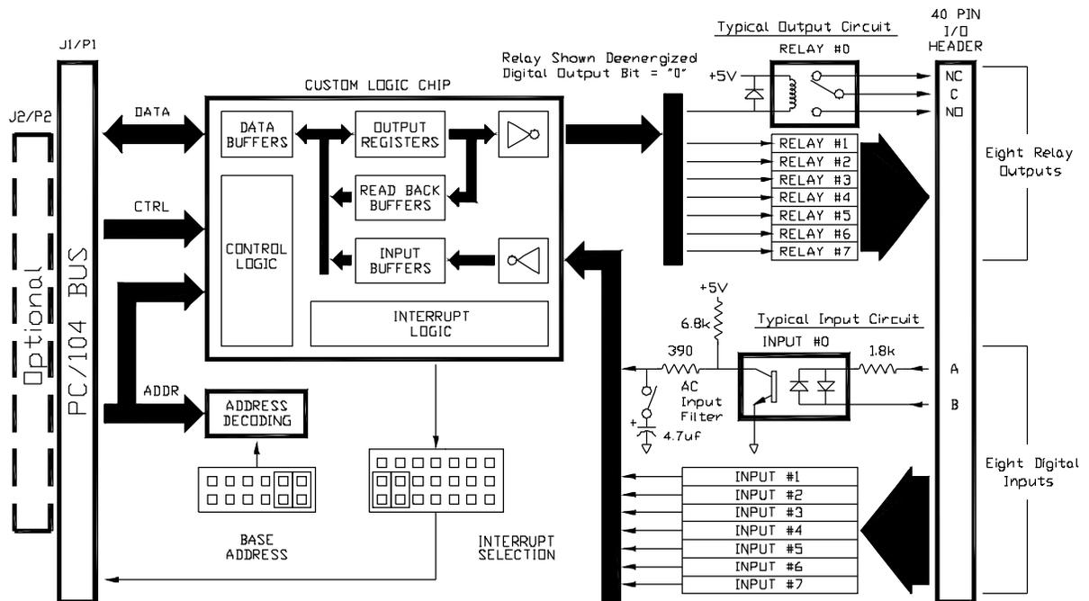
Figure 1 - RELAYIO-104 Simplified Block Diagram
