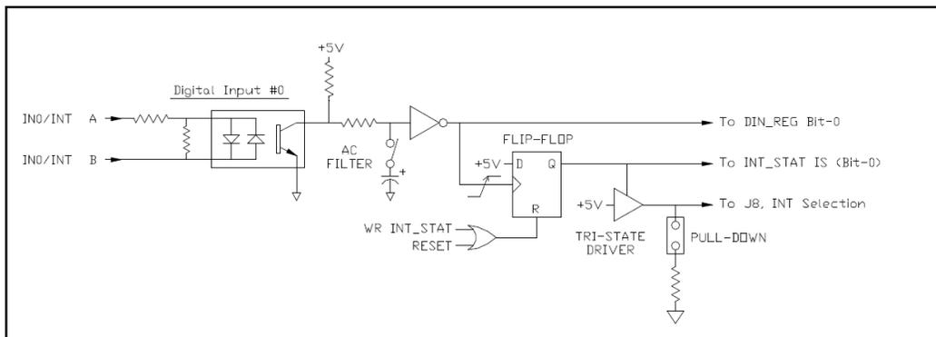
**Figure 6 - Interrupts Circuitry Block Diagram**
