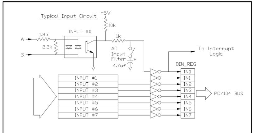
Figure 4 - DIN\_REG Functional Diagram
